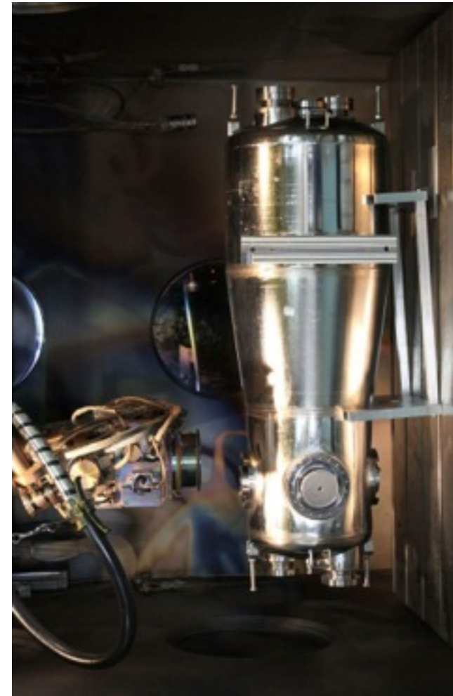
SCRF Cavity LHe Vessel EB Welding
