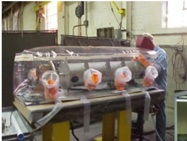
Welding a Titanium Pressure Vessel
