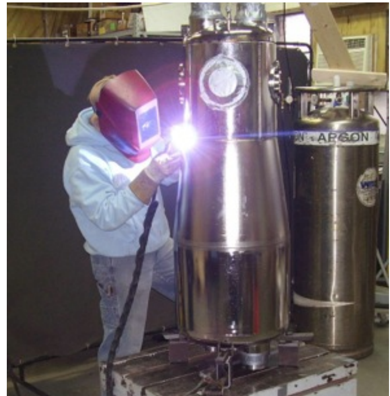
SCRF QWR Cavity LHe Vessel being welded at Meyer Tool
