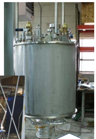
Cryostat Vacuum Vessel installed. Welded cylinder slipped over subassembly. Final test involve evacuation of the vacuum vessel and connected to a leak detector with the pressure circuits sequentially pressurized with helium gas.
