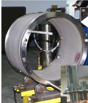
Two Cryostats in process. Liquid Nitrogen Vessel installed on left, Liquid Helium piping installed on right. Kapton tape on piping on right is part of temperature sensors' installation detail.
