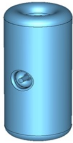
HWR - Type II 162.5 MHz - \beta \sim 0.24
