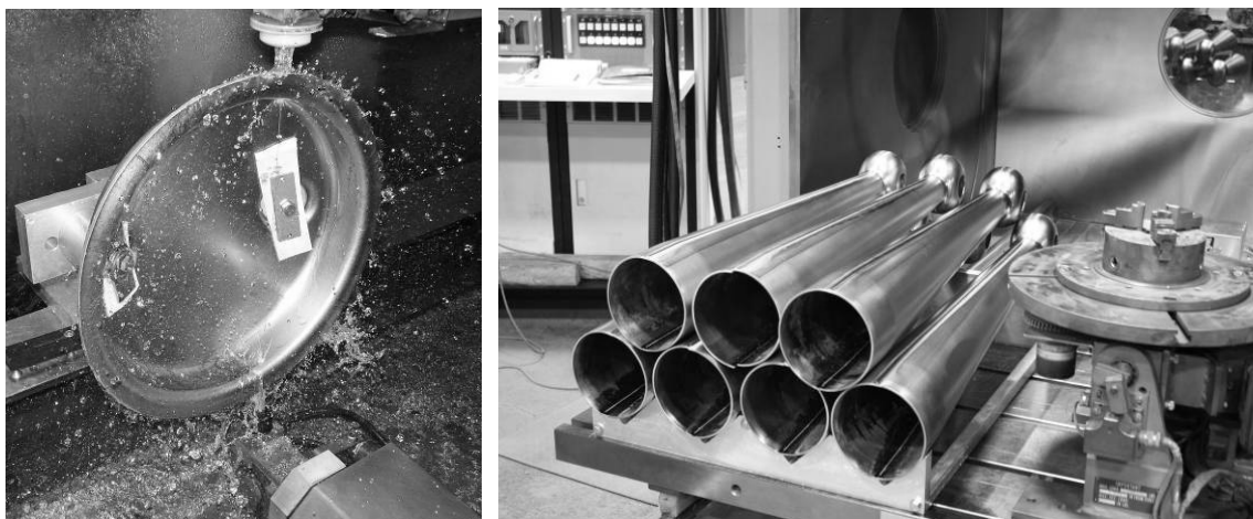
FIGURE 4. Wire EDM trim cuts are used to remove forming “flash” and to adjust part lengths for proper cavity frequency (left). Niobium parts are EB welded at Sciaky, Inc. using a library of weld parameters developed over the last decade by ANL in collaboration with Sciaky.
